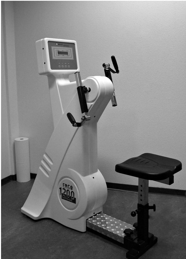
Figure 1: The arm crank ergometer (model Ergo-circle 1200) used in this study, from the company ERGO-FIT.
